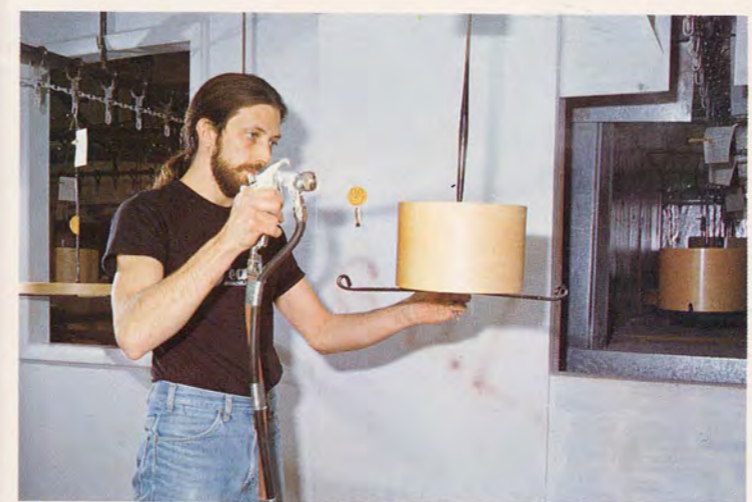
Spray booth with modern overhead conveyor system
