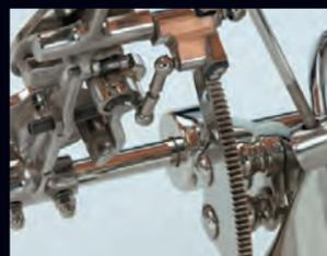
Precision gear driven pedal action. Schnelllar base is chrome vanadium steel for strength and durability.
